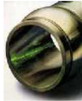
Liquid Penetrant Inspection
